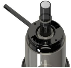
**Figure 6: Quartz Sleeve Installation**
