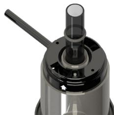
**Figure 6: Quartz Sleeve Installation**
